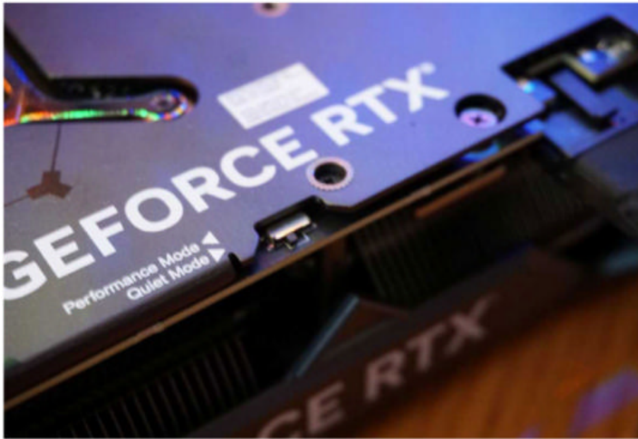
Asus includes a handy dual-BIOS switch on the Tuf.
