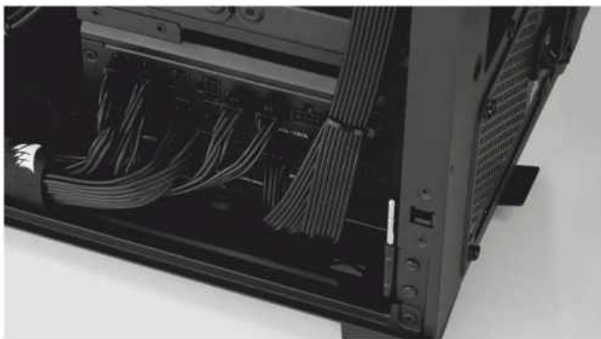
Corsair's RMx Shift power supply line rotates the conventional position of the power supply 90 degrees.
