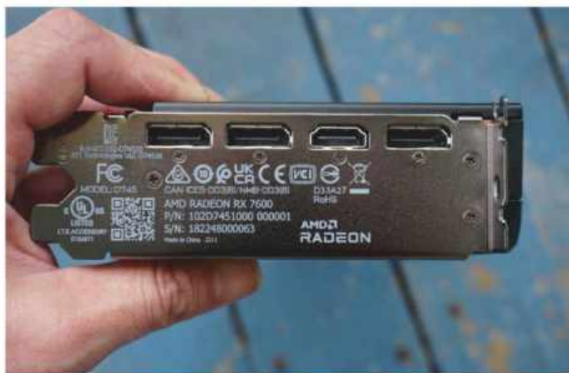
The reference card packs a single HDMI port and three of those speedy DisplayPort 2.1 connections.
