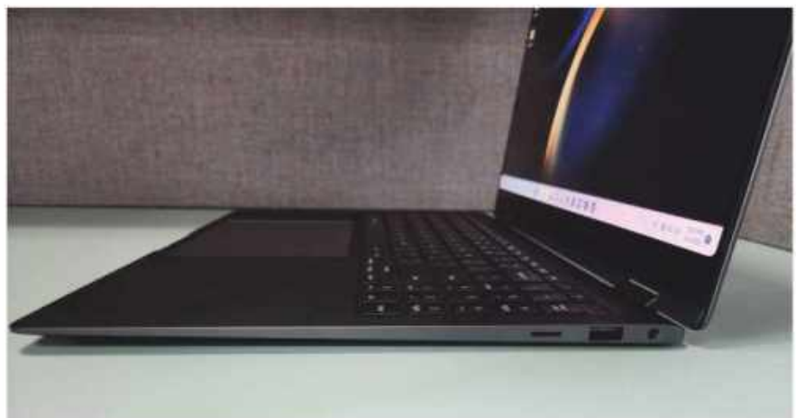
On the right side of the Samsung Galaxy Book4 is a microSD slot, a legacy USB-A port, and a headphone and mic jack.
