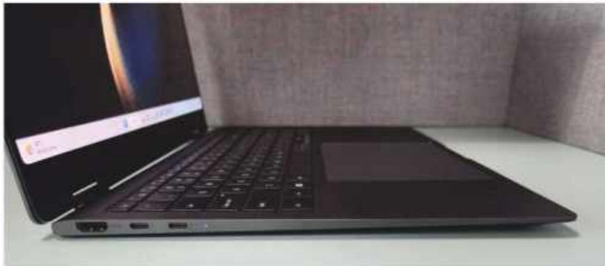
The Samsung Galaxy Book3 side ports include HDMI 1.4 and a pair of Thunderbolt 4 ports.
