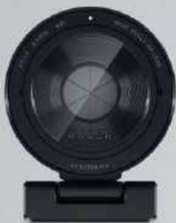
Rotate the frame counterclockwise and the built-in privacy shutter closes.
