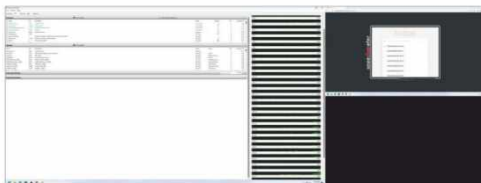
Chrome operating without a game open—both of the 7950X3D's processor dies are active and the tasks are going to the unstacked die first.
