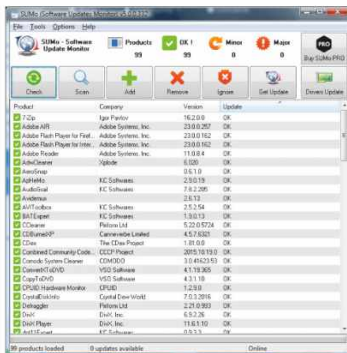
The Sumo update manager determines the version numbers of installed programs and compares them with its database to detect outdated software.
