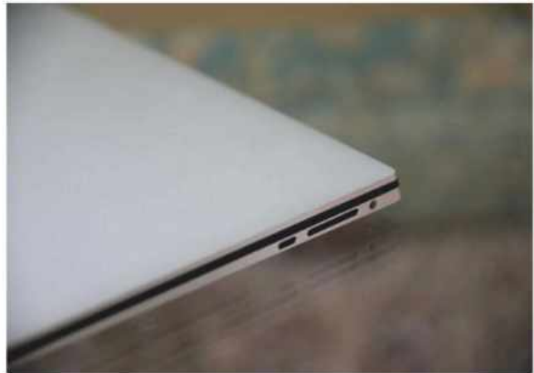
As well as three USB-C ports, the XPS 15 (2023) has a full-size SDcard reader and a 3.5mm audio jack.
