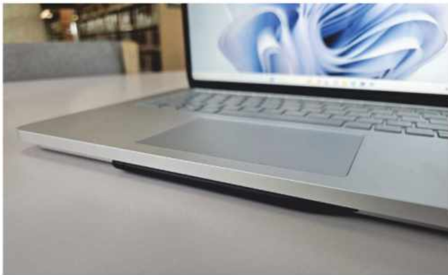
The (optional) Surface Slim Pen 2 sits underneath the Surface Laptop Studio 2, in a special cubby that also charges the pen.
