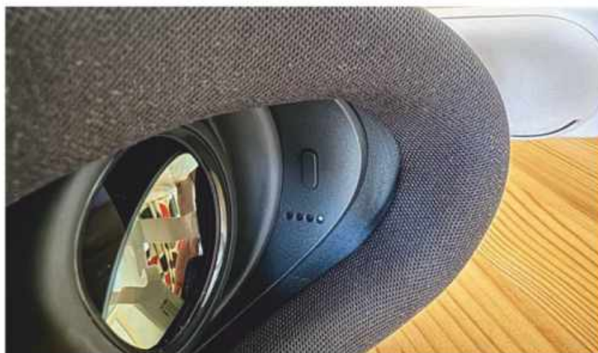
Buttons on either side of the headset allow you to adjust the distance of the lenses from your face.
