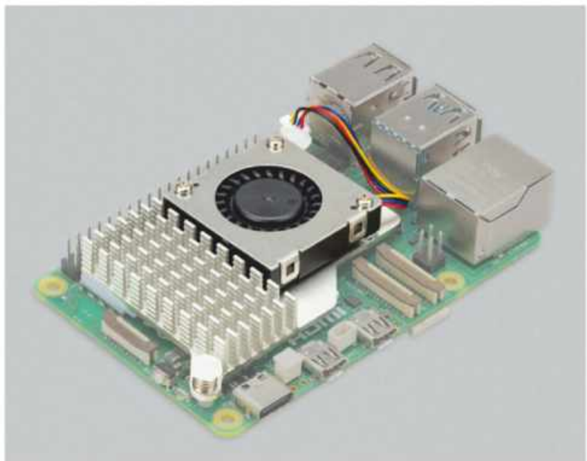
You can now cool the processor in a Raspberry Pi with an official active cooler.
