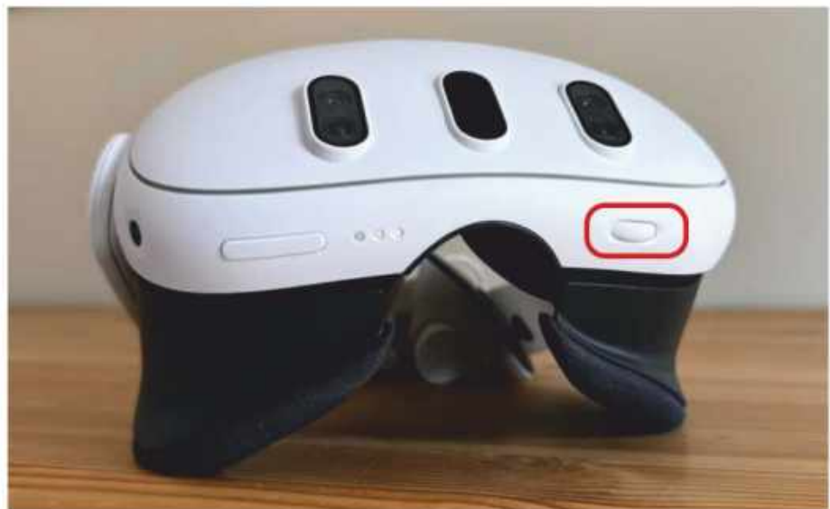
The IPD wheel (highlighted here) makes a welcome return, letting you adjust the interpupillary distance while wearing the Quest 3. The other button lets you control the volume.
