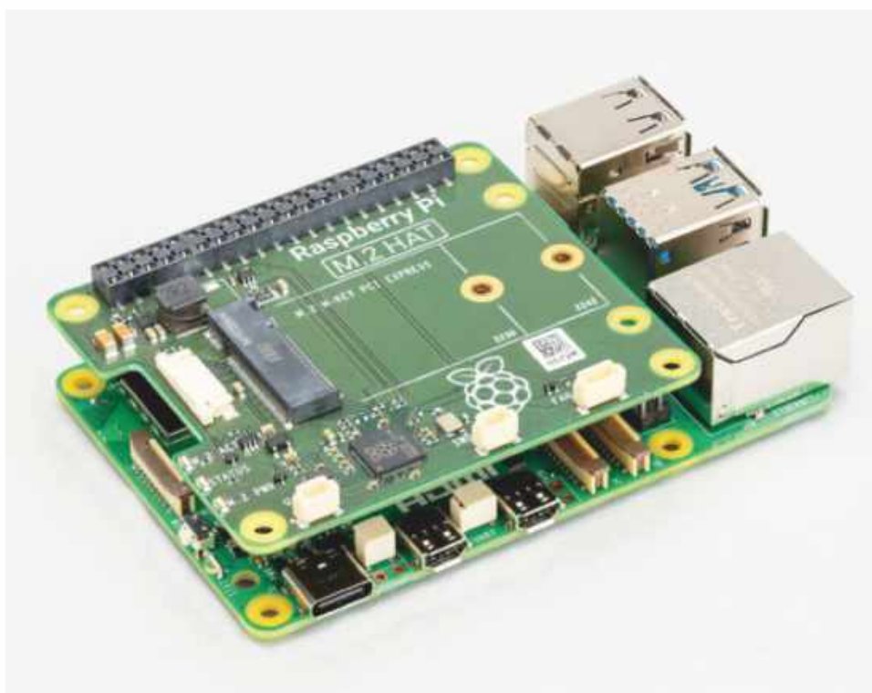
These M.2 HATs (hardware on top add-on boards) are new for the Raspberry Pi 5.
