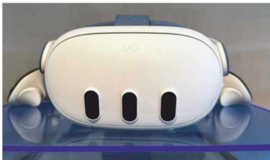
The most obvious change from the Quest 2 is the three pill-shaped protrusions on the front of the Quest 3.
