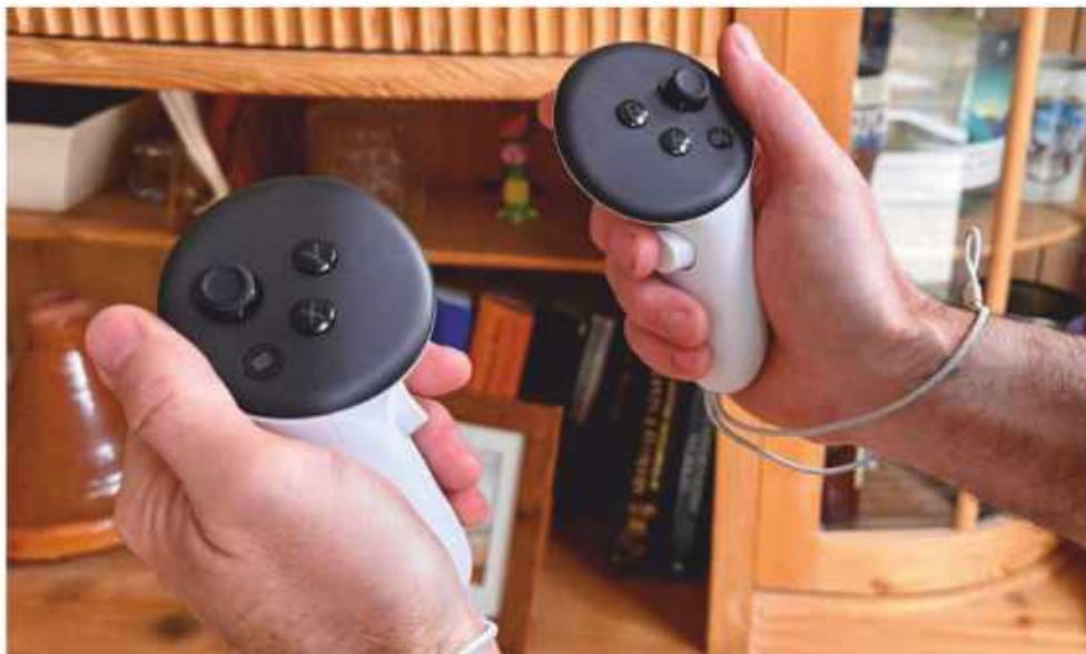
The Quest 3's controllers are more compact than the previous model's on account of not having tracking rings at the top.
