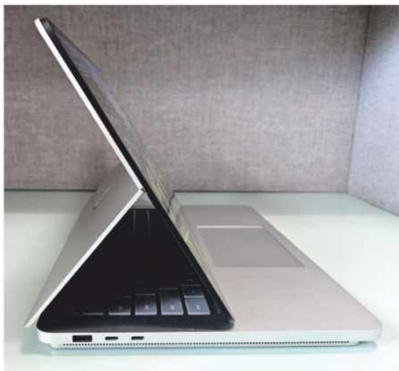
The Surface Laptop Studio 2's new USB-A port sits alongside the two existing Thunderbolt 4 ports. The display is in Stage mode, pulled forward.
