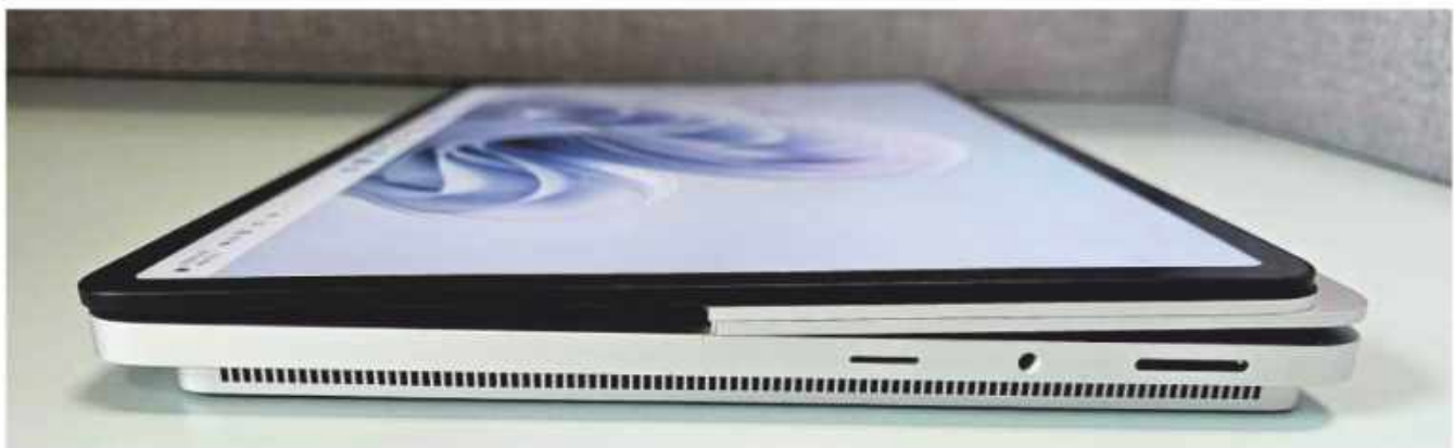
The Surface Laptop Studio 2, laid almost flat in Studio mode, for inking. A new microSDXC slot sits next to the headphone jack and the Surface Connector for charging.
