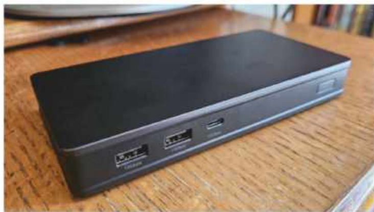
On the front of Ugreen's 9-in-1 USB-C dock are two 10Gbps USB-A ports and a USB-C port, too.
